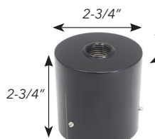
LF-AD-KNU 2" slip fitter adapter with 1/2" NPT hub in the top. Goes on 2" pipe and accepts a knuckle fixture.
